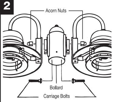
Attach each assembly from Figure 1, above to bollard base with carriage bolt, and plastic acorn nut.
