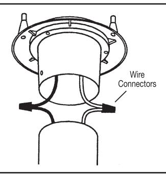
Connect the wires. Note: Attach black fixture wire to black supply wire, white fixture wire to white supply wire. DO NOT mix them up. Use wire connectors.
